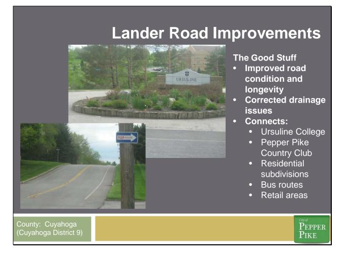
The Lander Road Improvements Project included replacement of all storm sewer and catch basins along Lander Road. Minor drainage issues along the road were identified and corrected. Base repairs were performed as needed along the project length, and a total of 2.6 miles of road were resurfaced. The final product is a safe, durable roadway complete with bicycle/pedestrian berm that will benefit the residents of Pepper Pike and its neighboring communities for many years.
